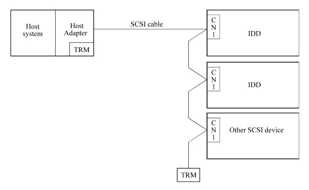
Figure 5.1 SCSI bus connections (1 of 2)
